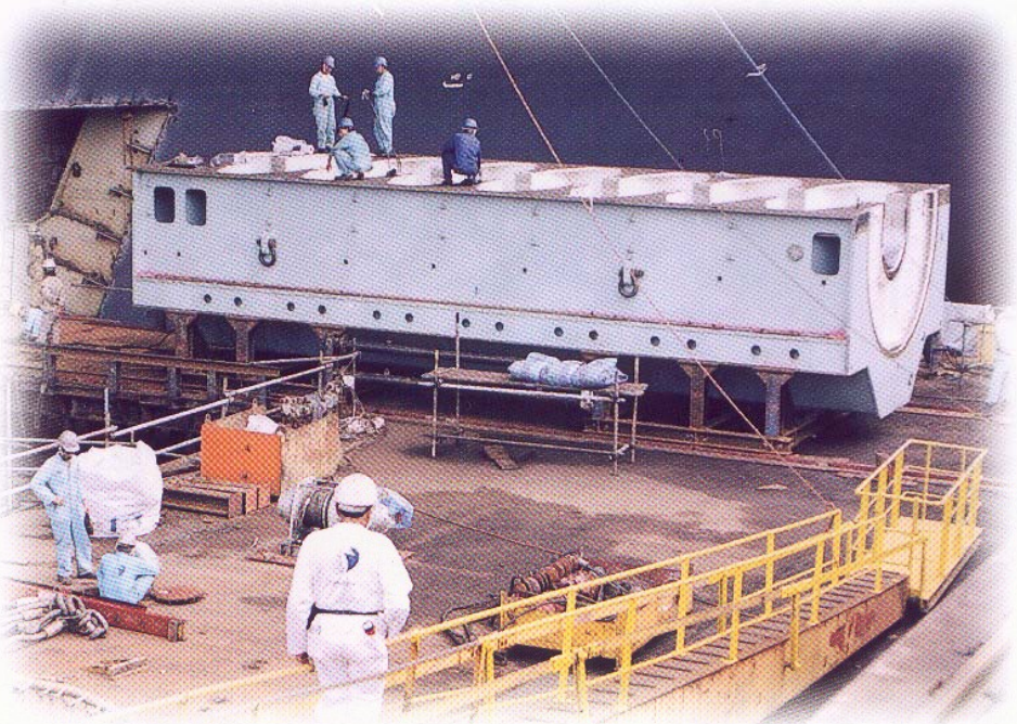
Final adjustments being made before the bedplate is repositioned in the main engine compartment
